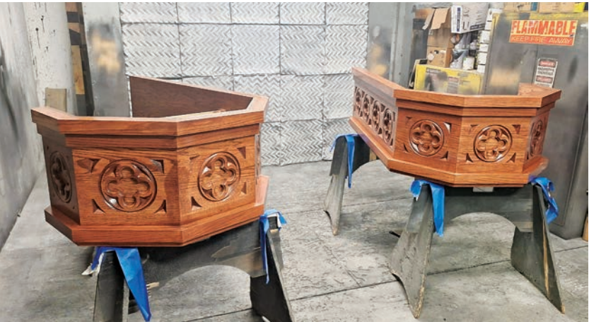
Elements of casework being finished in our spray booth
