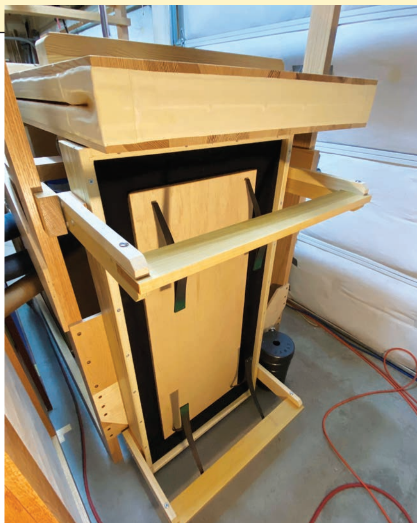
Figure 3: A floating concussion plate is mounted vertically at the back of the wedge bellows. The area of the floating plate is equal to the swept area of the wedge bellows (half of its total area), making the surge shallower and more stable.
