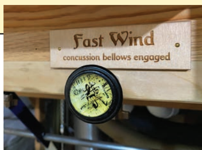
Figure 4: This knob activates a large pallet, engaging the floating concussion plate for a shallower surge.
