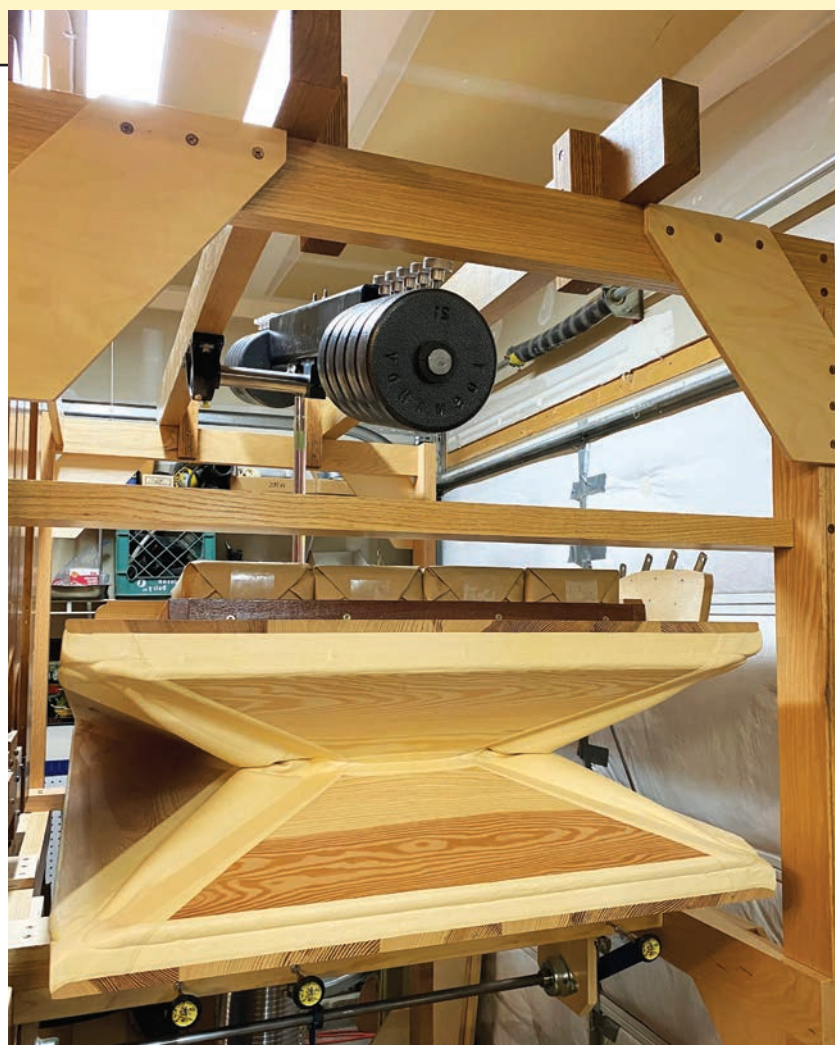
Figure 1: In the image at the left the blower is turned off and the wedge bellows is fully collapsed. The balanced beam above it is rotated upward at the front. The blower is turned on in the image at the right, and the wedge bellows is fully extended. The balanced beam above it is rotated downward at the front. Playing a chord will make the bellows drop, and the beam will rotate upwards. The balanced beam in these images has the full complement of mass with 50 kilograms (110 pounds) at each end of the beam, producing the slowest wind surge. The attachment point of the connecting rod to the balanced beam is one fourth of the distance between the center of the beam and the center of the mass at the back end of the beam; this produces an effective inertia of 400 kilograms. The balanced beam is clamped to the shaft and rotates in the bearings at the sides. Removing mass in equal amounts from each end of the balanced beam will make the wind respond faster. Figure 2 (see page 18) shows the length of the surge response with different amounts of mass on the beam.
