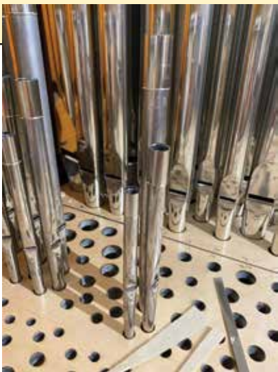
Figure 14: Voiced and tuned pipes of the three-rank Fourniture, one of three mixtures on this windchest
