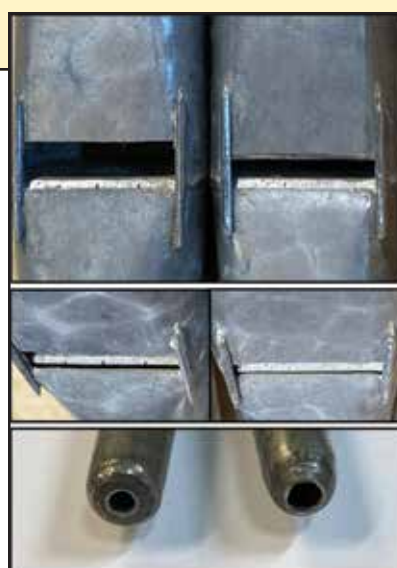
Figure 20: The pipe at the left has a higher cutup (top), a generous flueway depth (middle), a lower 0.63 toe constant (bottom), and produces fast speech. The pipe at the right has a very low neo-Baroque cutup (top), a very constricted flueway (middle), a much more open 1.29 toe constant (bottom), and produces slow, gulping speech.
