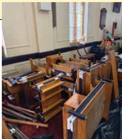
Skinner Organ Company Opus 635, Hazelton, Pennsylvania, eight reservoirs and two tremulants (photo credit: John Bishop)
