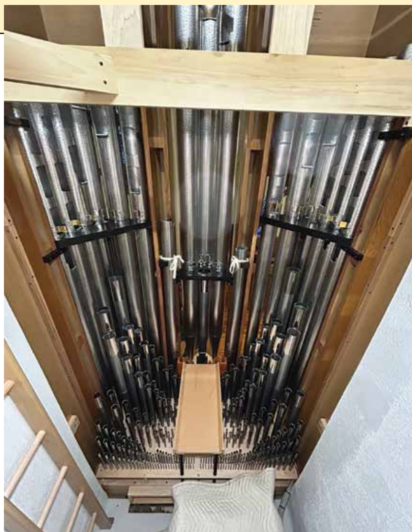
The Great division is entirely contained within the case, which is less than five feet wide and three feet deep.
