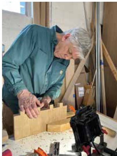
Bart Dahlstrom hand cuts dovetails in the rift-sawn white oak for the case impost.
