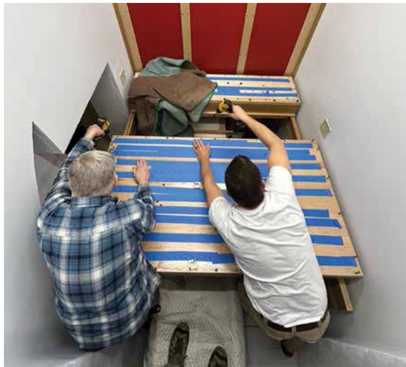
Bart Dahlstrom and Dave Mitchell work to install the main Swell chest. The Swell chamber, home to seven stops, including a full-length 16' reed, is only about 5'6" by 6'6". Creative engineering was necessary to make everything fit and be reachable for maintenance.
