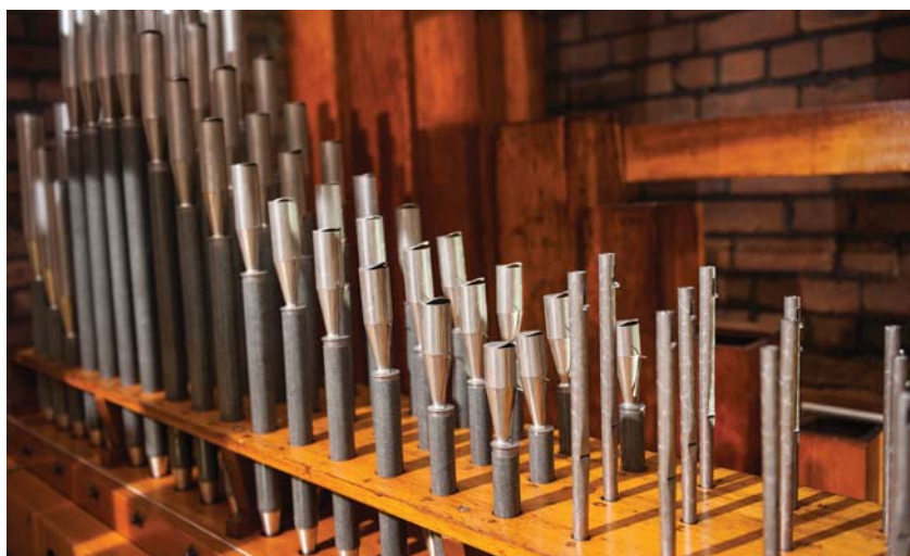
Reconditioned Vox Humana chest and pipes (photo credit: © 2014 David Ottenstein)
