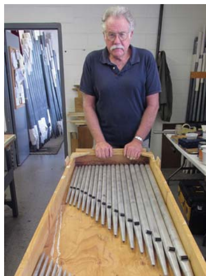
Nicholas Thompson-Allen with the freshly cleaned and regulated pipes of the Dolce Cornet (photo credit: Thomas Murray)
