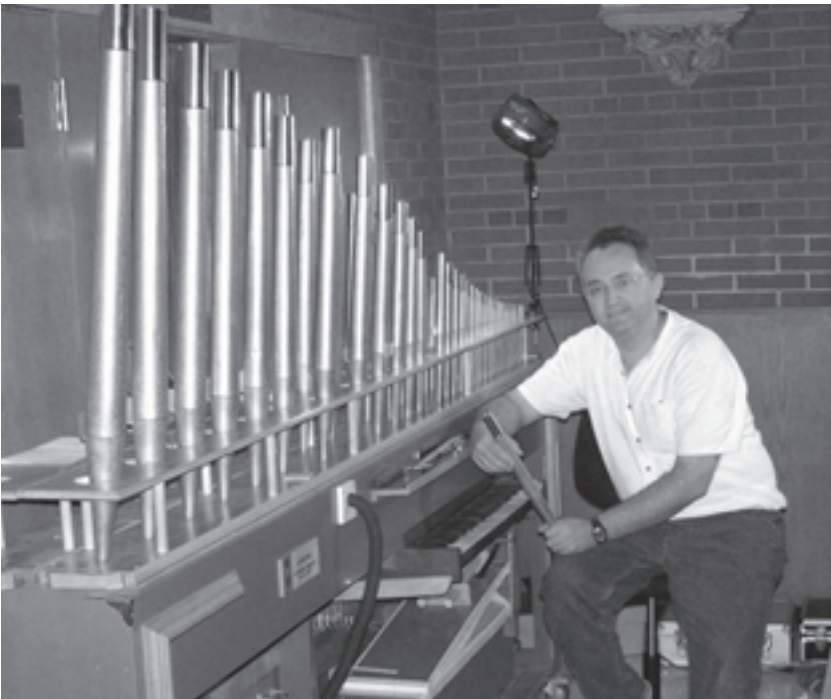
Voicing in progress—Tomasz Lewtak at custom-built voicing organ
